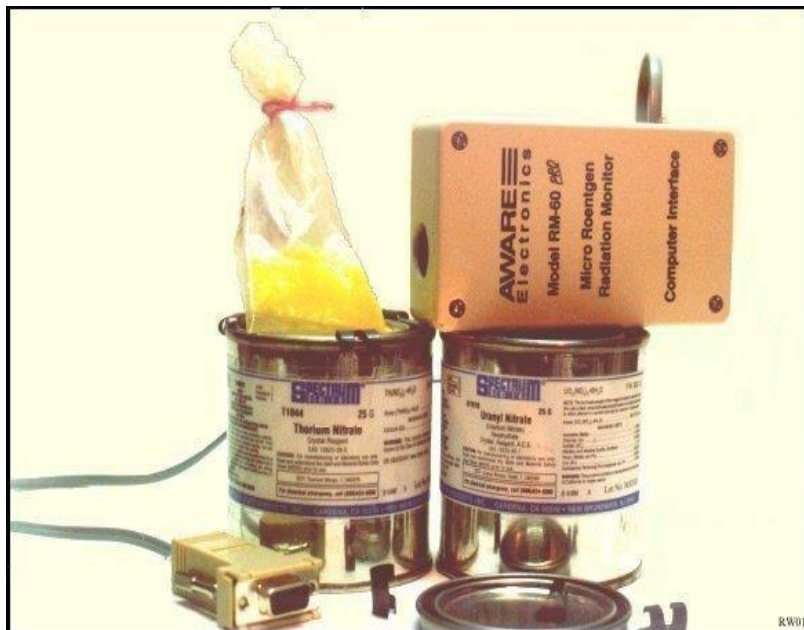
These are the basic materials and tools required for these experiments. The yellow crystals in the plastic bag are uranium nitrate hexahydrate, but most experiments can be done with the safer thorium nitrate tetrahydrate. The RM-60 counter connects with a computer through the serial cable.
