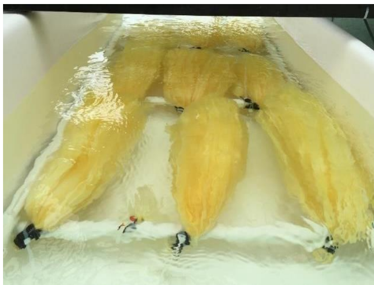
"Material designed to capture uranium from seawater as an alternative to land-based mining of the fuel for nuclear power production is tested at PNNL's Marine Sciences Laboratory. Credit: PNNL"
