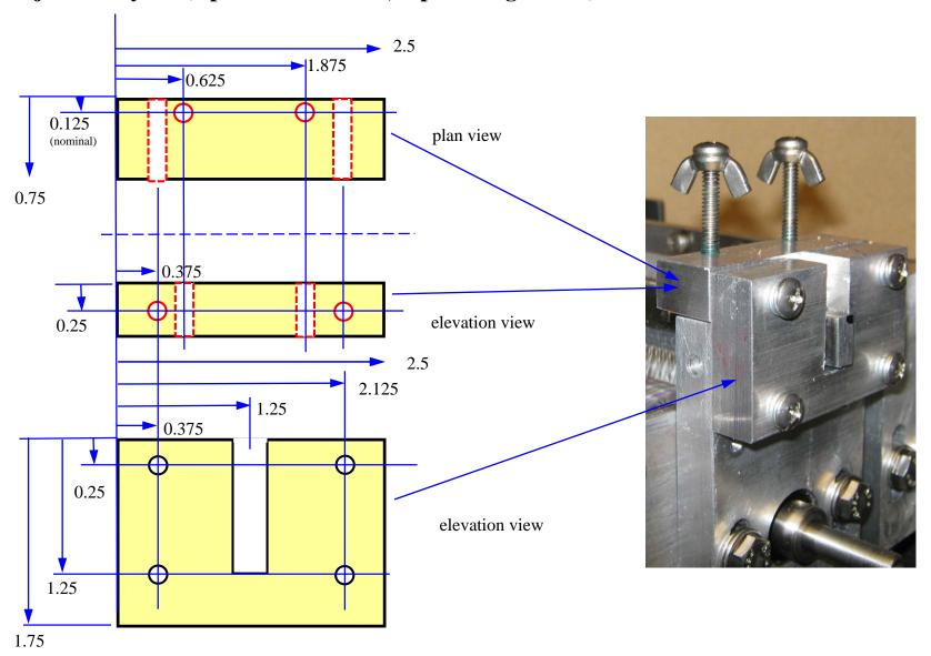
Red holes are tapped for 10-24 screws. Blue holes are 3/16" pass-thru. Upside down wing nuts are secured with high strength thread locker (red). Adjusting screws are treated with a small drop of medium strength thread locker (blue) to prevent rattling.
