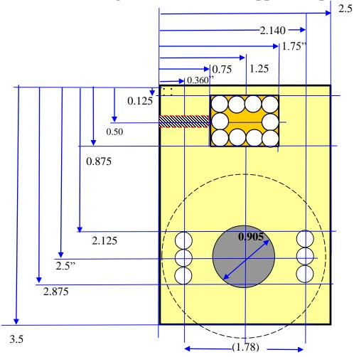
Screw holes (slots) are to pass ¼-20 Allen screw Use 19/64 drill for holes and webs to emulate a milled slot. File smooth.
