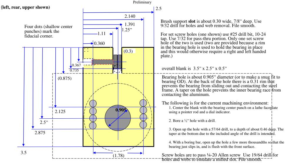
Fasteners used in each slot are ¼-20 stainless Allen head screw with one wave washer (1/4") and two #12 stainless flat washers.
